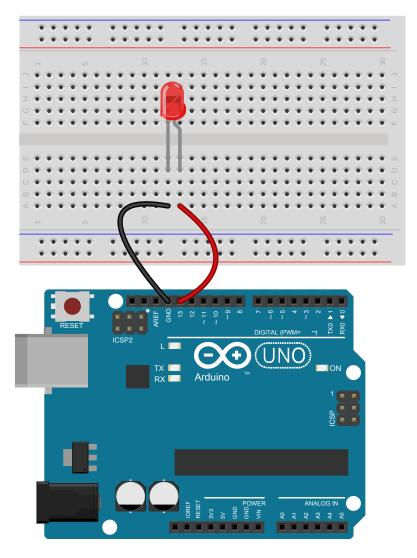
Now, connect the Arduino to your computer using a USB cable. Here's the code that will flash your light. Type it into the "Arduino" software you can find in the "ClassFiles" folder:
